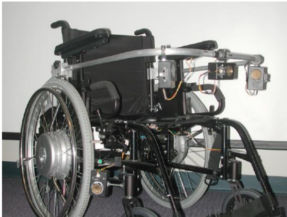
Slika 7: The Smart Power Assistance Module - SPAM (Sampson, 2005)
